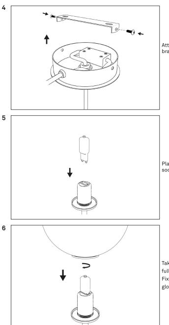
Attach the ceiling plate to the bracket with the screws.
