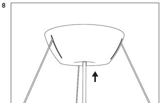
Attach the cover plate to the mounting plate by carefully sliding cover plate up and let the magnets fixate it.
