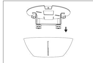
Remove the cover plate from the mounting plate by pulling them apart by hand.
