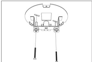
Fixate the mounting plate to the ceiling with screws.
