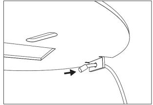
Lead the three wires through the holes in the mounting plate.
