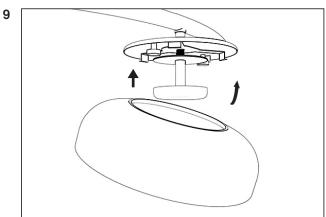
Attach each glass by fixating them with the three hooks located inside each of the 8 lamps.
