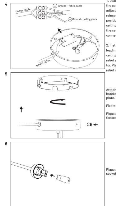
1. Lead the fabric cable into the cable connector. NB: After adjusting the length carefully reinsert the cables in same positions: Ground cable from ceiling plate and ground cable in the center of the cable connector.
